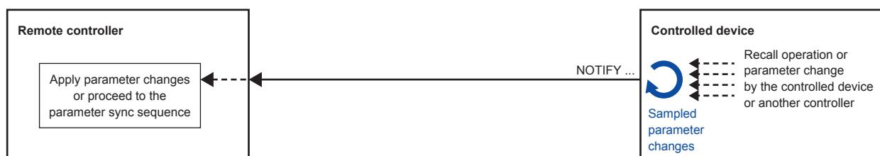
The way in which parameter change notifications are sent varies depending on the value notification mode specified in the MTX external control protocol mode.
