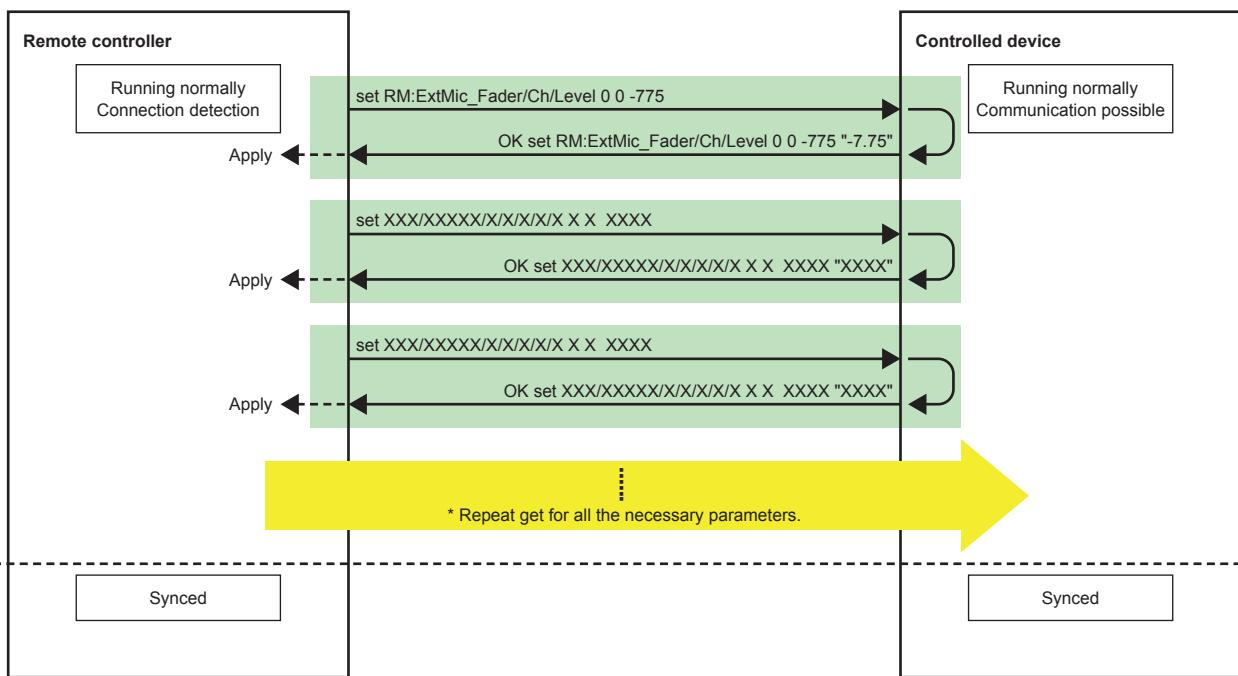
Even when the latest state on the controller side is reflected, depending on the situation, the value may be rounded on the operation target device side.
