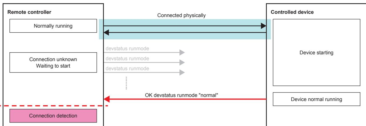
Example when the controlled device starts earlier than the controller
