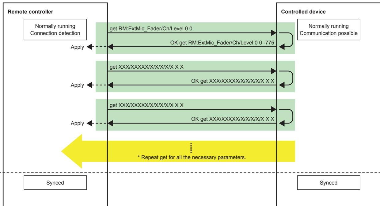
Executing this sequence synchronizes the status with the controlled device.
