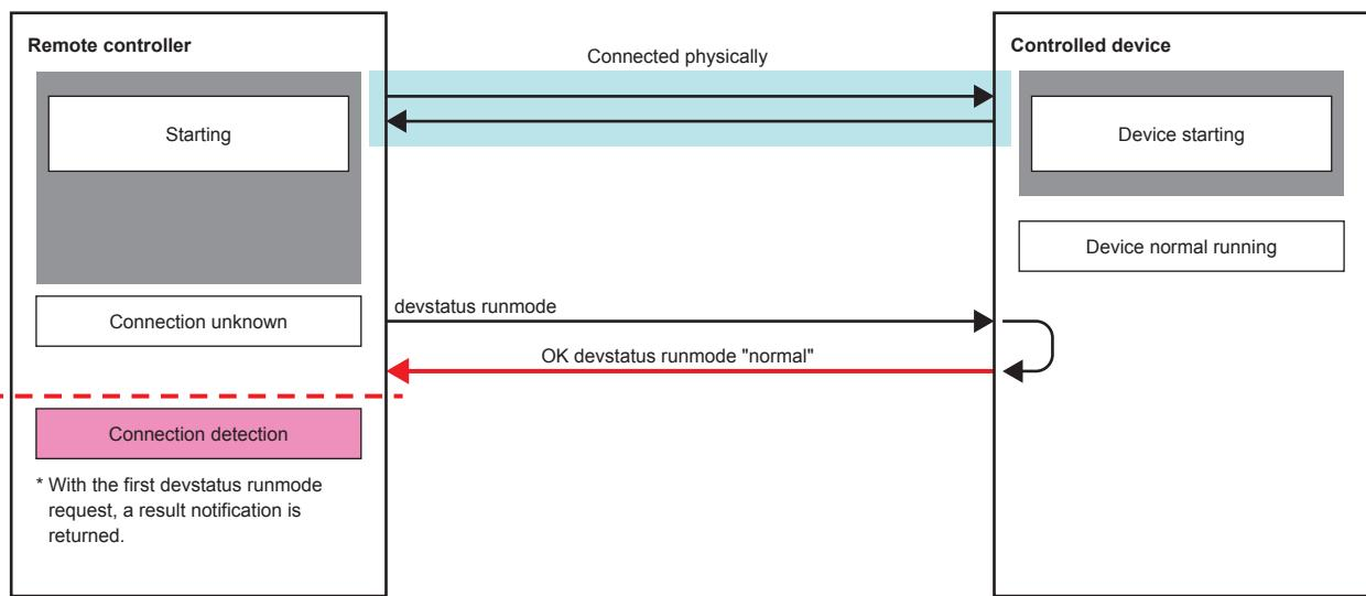
Controller can recognize that Controlled device is ready to receive commands when there is response for "devstatus runmode" command.
