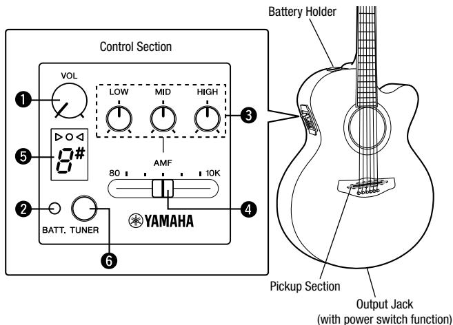
The built-in preamplifier is automatically turned ON when a guitar cable is connected to the output jack.
